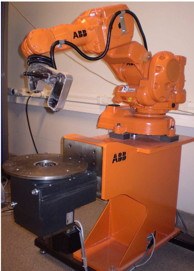
Fig. 2. The laser profile scanner mounted on an industrial robot equipped with a turntable.
